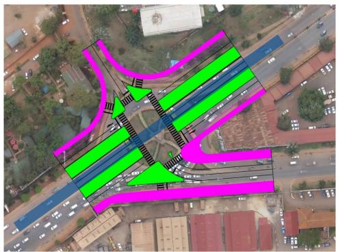
Figure 2-4: Hotel Africana Roundabout after the project with BRT (in Blue) in place with capacity of about 7,422 pcu/hour
