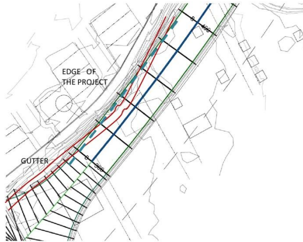
Figure No. IV.17. Detail of old gutter left behind by abandoned hydroelectric plant.
