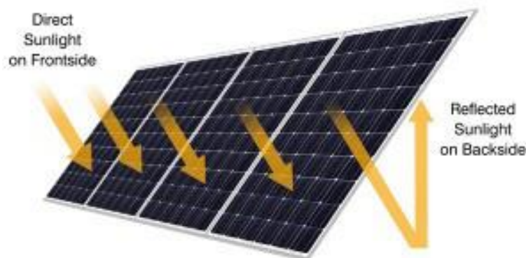
Figure 2-7: Typical Bifacial PV module
