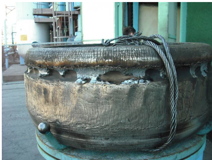
Fig.4.2-11 Mill Roller before Maintenance
