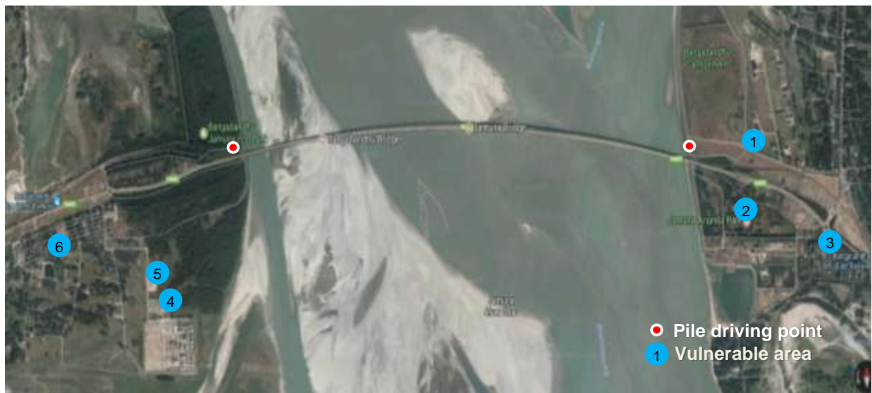
Figure 6-4 Pile driving points and Location of Vulnerable Areas
