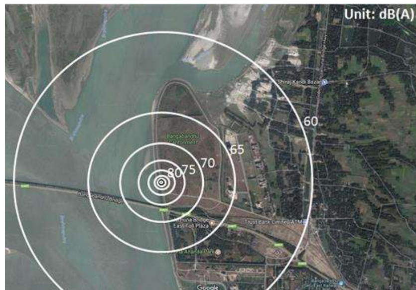
Figure 6-2 Result of Noise prediction by Pile driving on the east riverbank of Jamuna River
