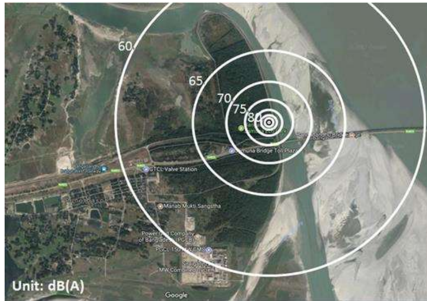
Figure 6-1 Result of Noise prediction by Pile driving on the west riverbank of Jamuna River
