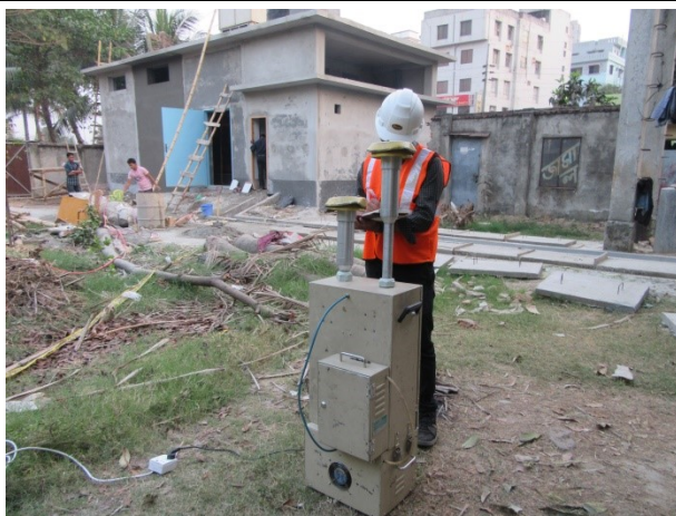
AQ5-3: Air Quality Monitoring at Mirpur 10 Station
