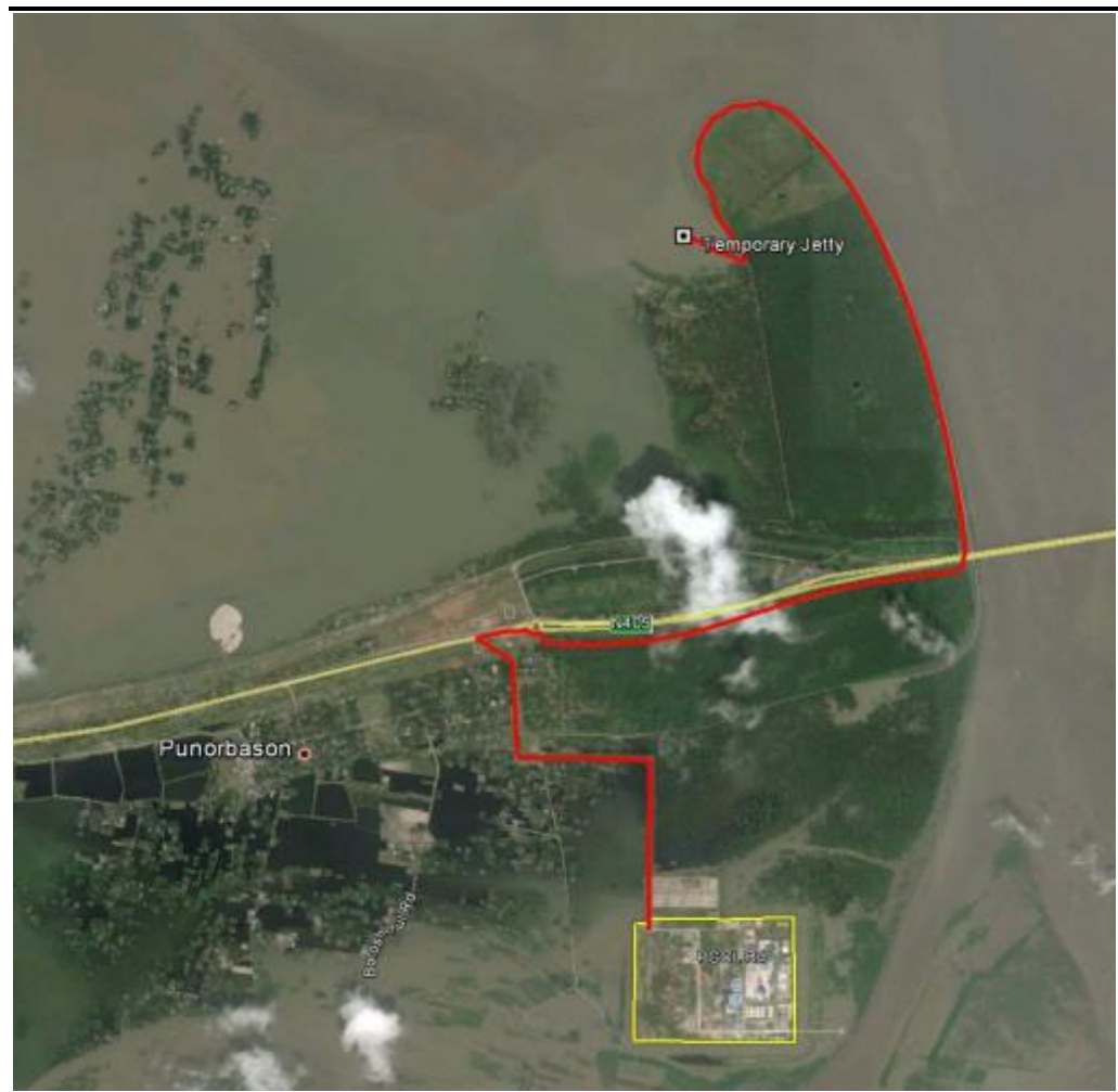
Figure 3.15 Location of Temporary Jetty and Heavy Lift Movement Route
