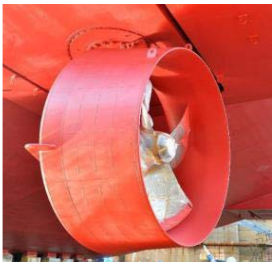
Figure 2.5-41 Example of Azimuth Propeller
