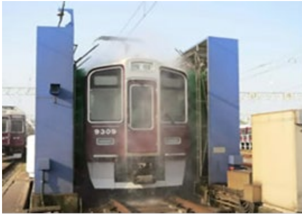
Figure 4.10.3 Example of automatic rail car washing machine
