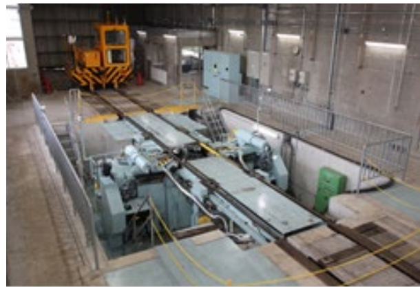
Figure 4.10.4 Example of Wheel surface grinding machine for wheel truing
