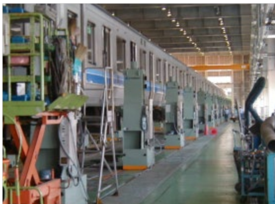
Figure 4.10.5 An example of the device which can inspect and maintain the parts by lifting all the car bodies at the same time
