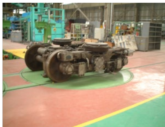
Figure 4.10.6 Turntable for the bogie
