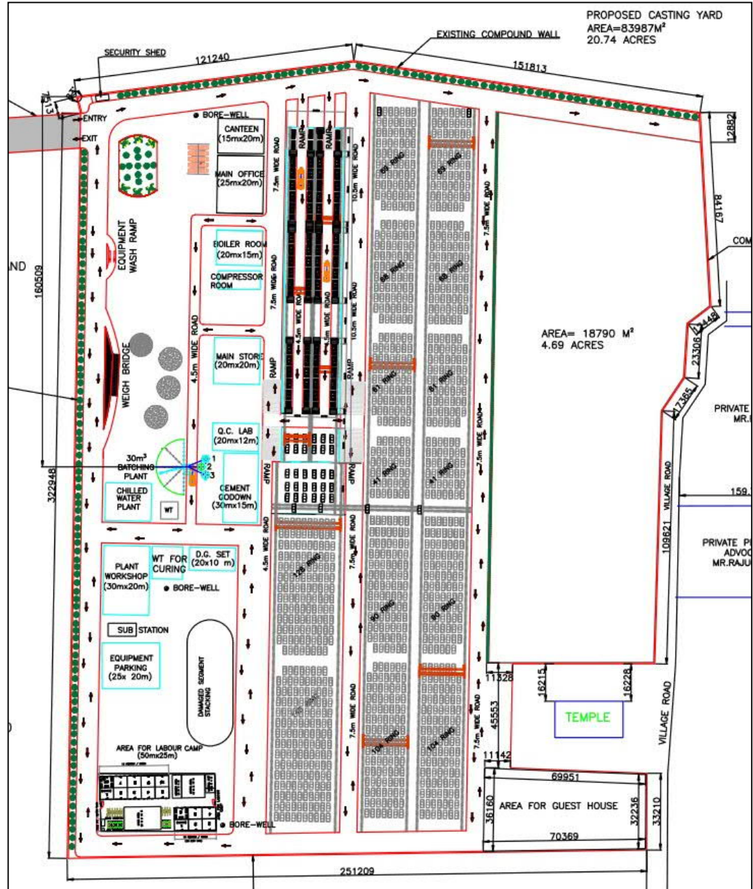
Figure 2.2: Typical Casting Yard for two Packages
