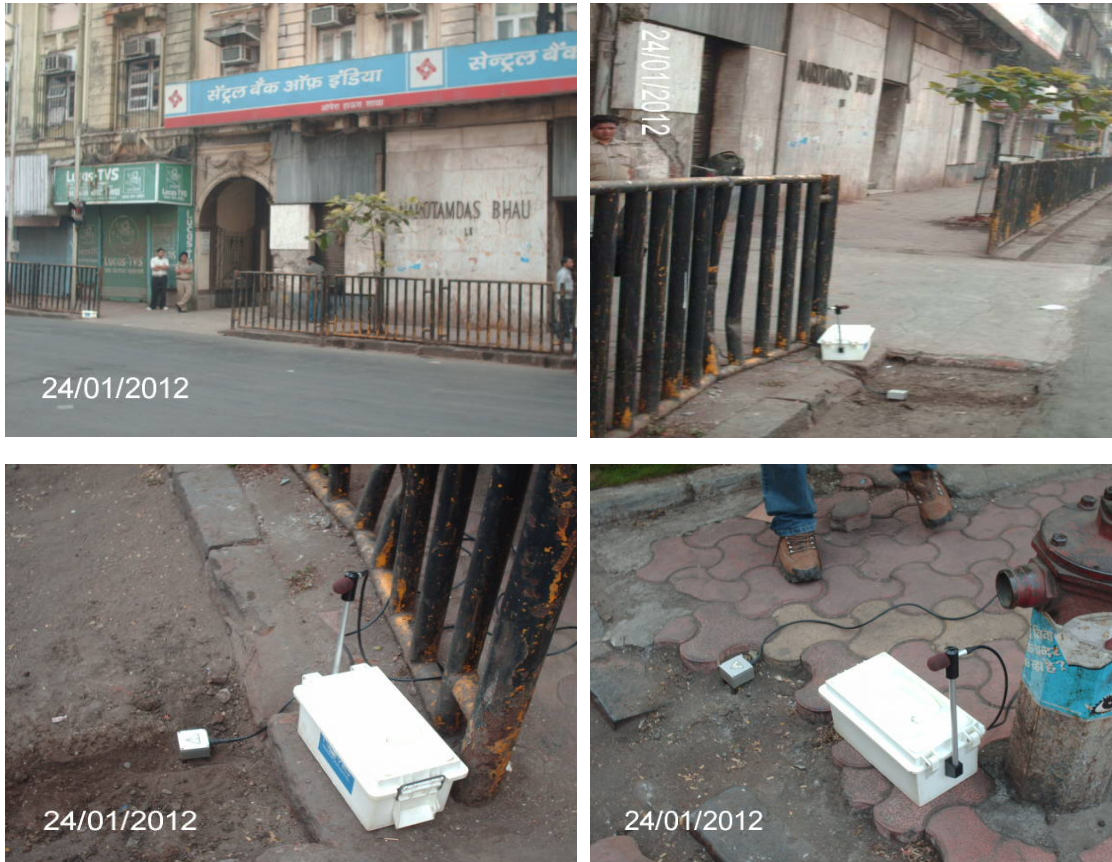
FIGURE 3.33 VIBRATION MONITORING AT LOCATION LAMINGTON ROAD
