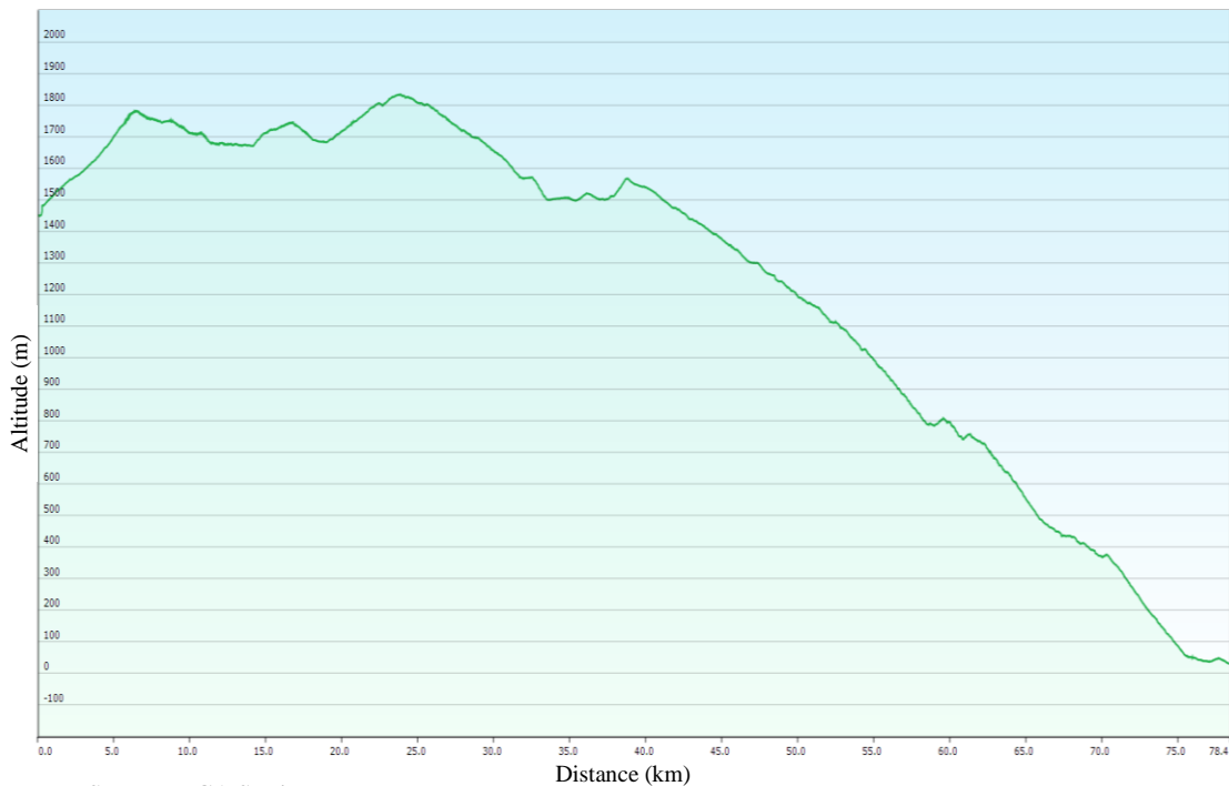
Figure 3.2.10 Existing Road Profile of NH40
