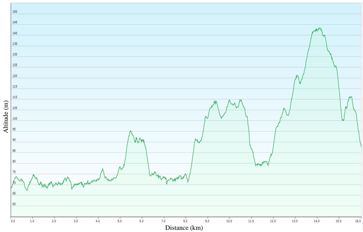
Figure 3.2.17 Existing Road Profile of NH44A (Manu Side)
