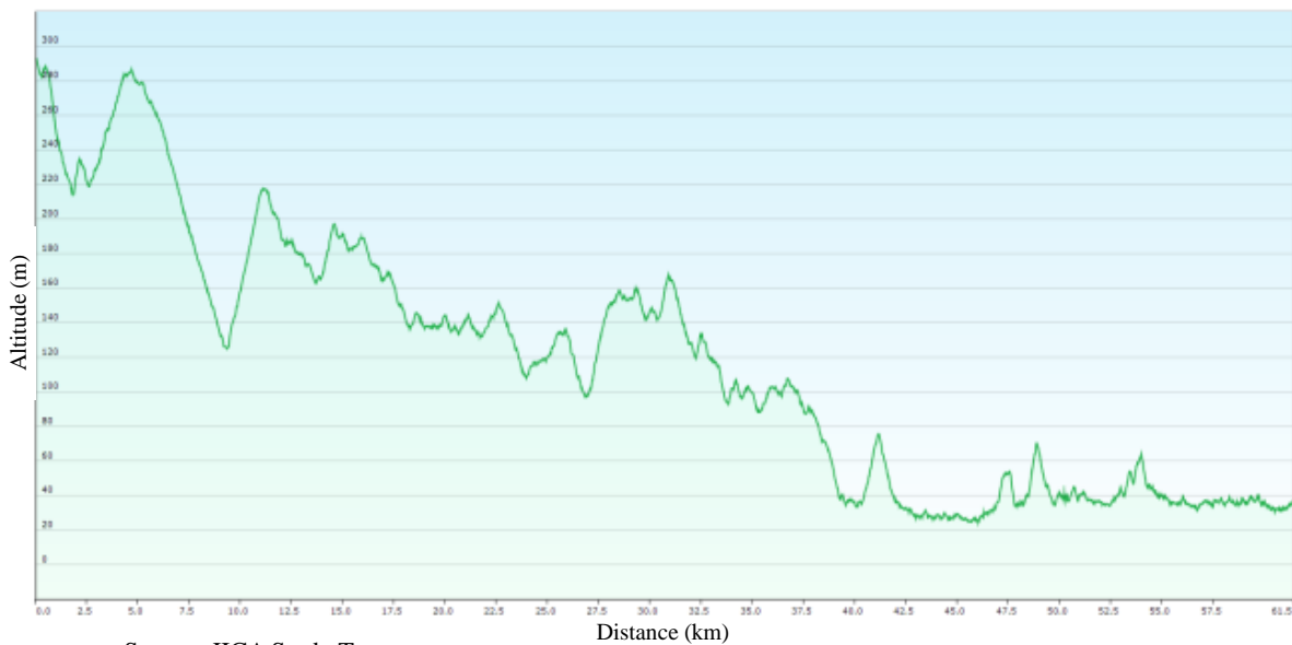
Figure 3.2.7 Existing Road Profile of NH51
