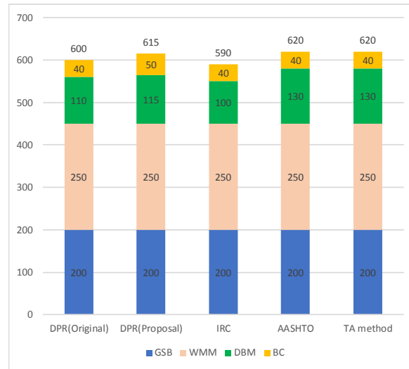
Pavement thickness of section 2 (case 1)
