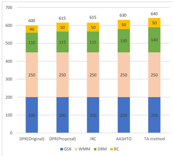
Pavement thickness of section 1 (case 1)
