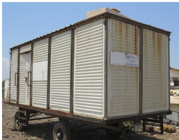
Photo 4.c: Mobile Asbestos Decontamination Unit
