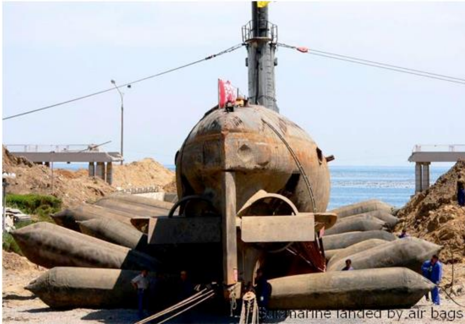
Photo 5.f: Decommissioned Submarine Being Raised on to Dry Land over Air Bags for Scrapping
