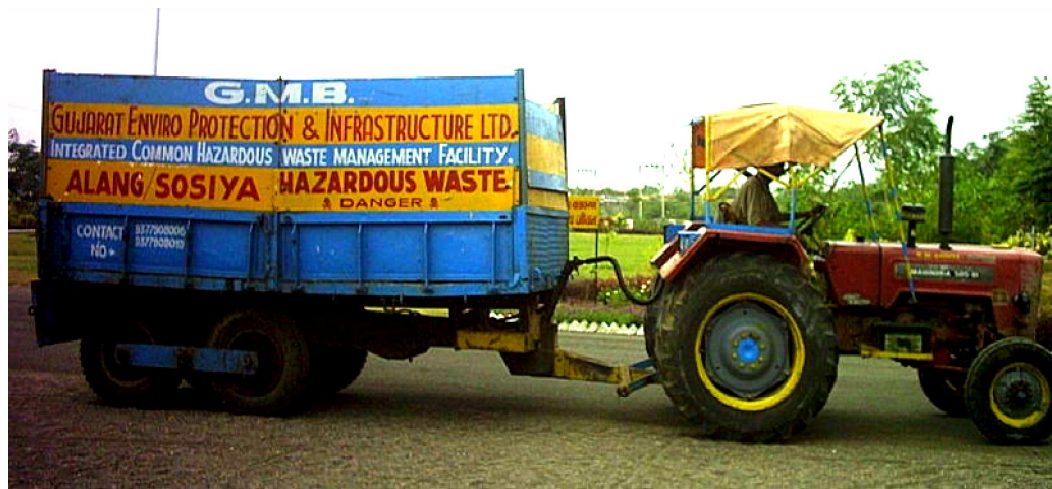
Photo 4.f: Dedicated Tractor Trolley for Transportation of Hazardous Wastes from Plots to Alang TSDF
