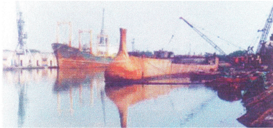
Photo 5.d: Ship-breaking at Khidderpur Dock, Kolkata by Berthing. Ship on the right partly broken up, the one on the left waits its turn
