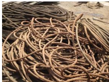
Lack of routine check of fixtures including winch line (Normal yards)
