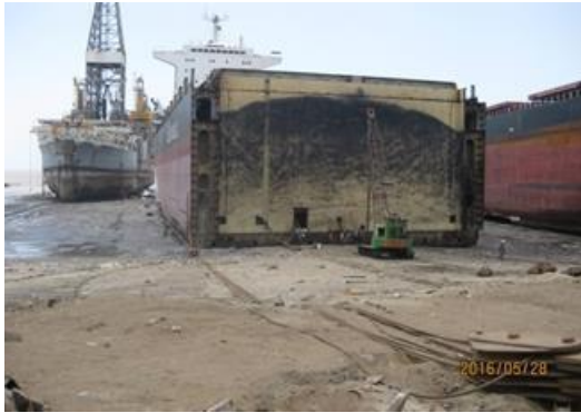
P.V-7 rear half of hull body to be dragged
