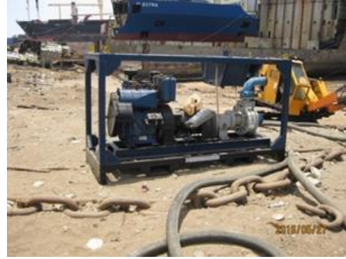
P.V-5 Mobile fire pump
