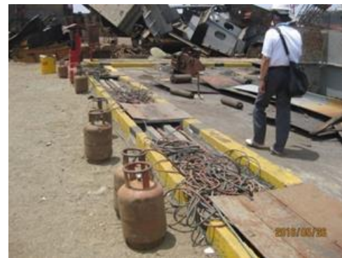
P.5 fixed supply pipe of oxygen gas and LPG gas bottles
