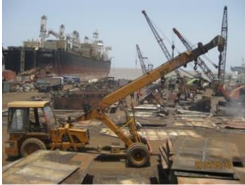
P.68 wheel crane distributing plates
