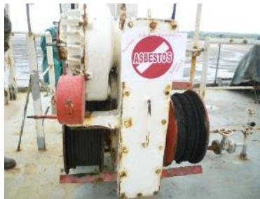
Identification of hazardous substance including asbestos on board (NK certified yard)
