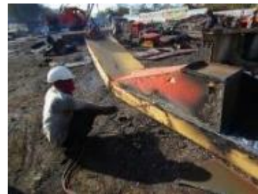
Wearing cloths instead of mask during gas cutting (Normal yards)
