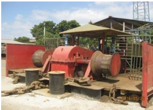
P.78 75 t Winch with fence
