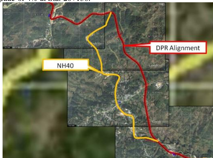
Figure 5-107: Existing NH40 and Proposed Alignment of Bypass #4
