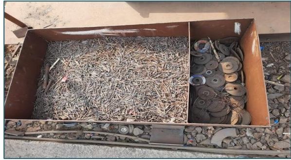
Welding butts & cutting wheels are stored in metallic bin, Metal scrap used to make Box for collecting nails at Ch 268 store
