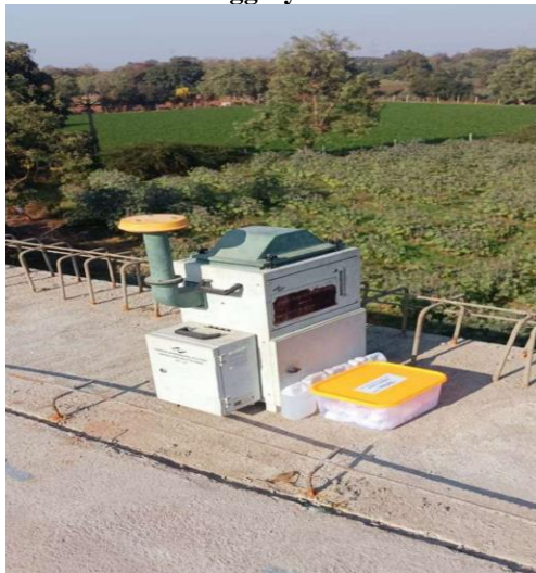
Ambient Air Monitoring device installed
