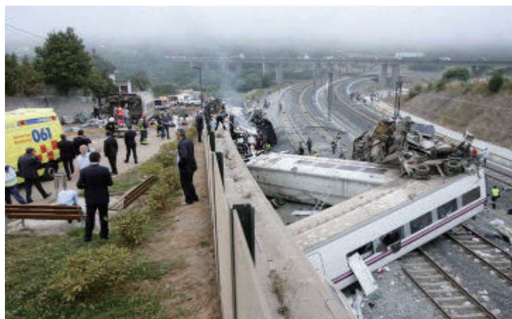
Figure 4.4-2 Overturn Caused by Over Speed on a Conventional Line
