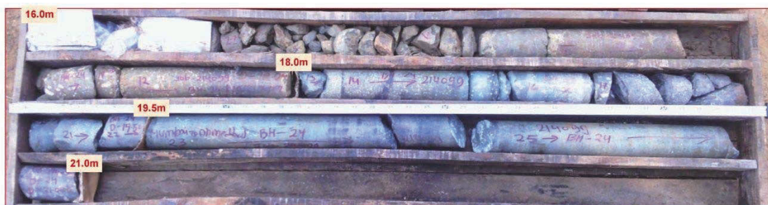
Figure 6.2-30 Photograph of Rock Core Sample (BH-No.24)
