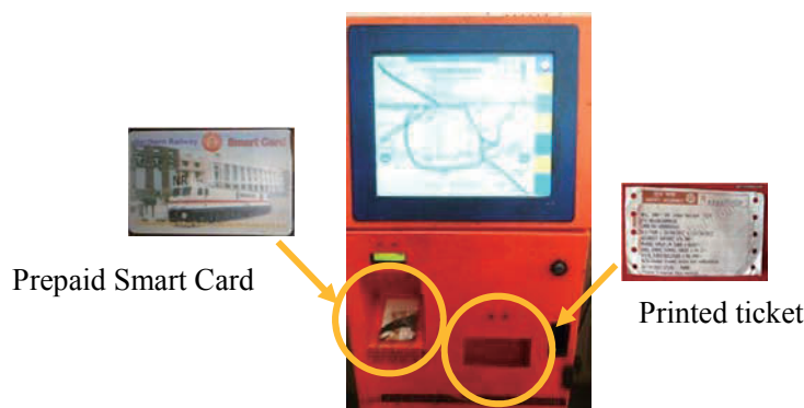
Figure 9.13-8 TVM used for the Existing Railways
