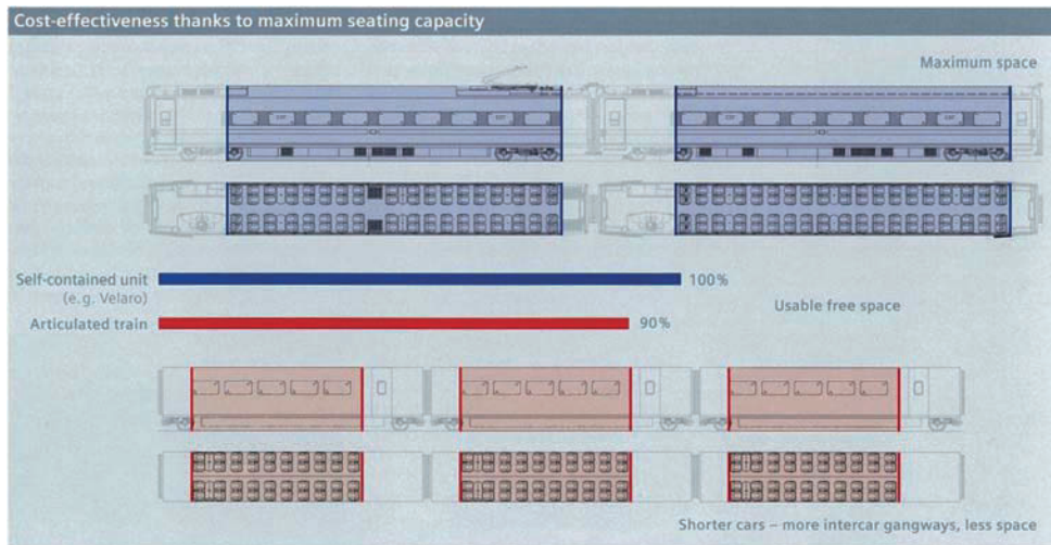
Figure 9.8-1 Comparison of Non-articulated and Articulated Bogie System
