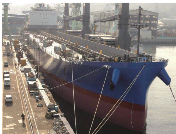
Figure 9.7-38 Long-Rail transporting Ship (Source: Sumitomo Corporation)
