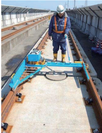
Figure 9.7-73 Measurement with a Track Master Figure 9.7-74 Rail Fastening
