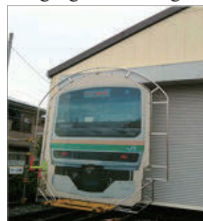
• Clearance gauge and rolling stock gauge
