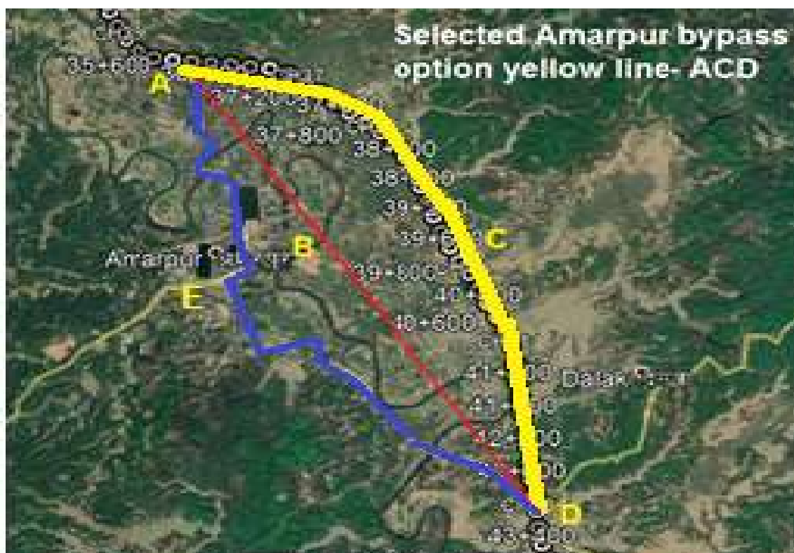
Figure 3.5: GIS image of Alternative Alignment Option Study for Amarpur Bypass
