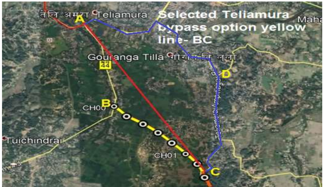
Figure 3.2: GIS image of Alternative Alignment Option Study for Teliamura Bypass
