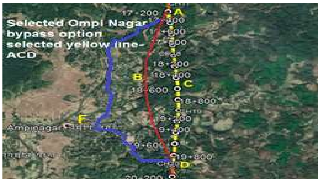
Figure 3.4: GIS image of Alternative Alignment Option Study for Ompi nagar Bypass
