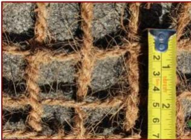
Coir geo-textiles specifications: Grade I- 400g/m 2
