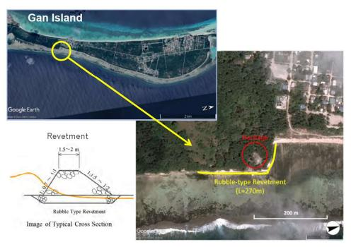
Figure 5.4.12 Original Layout Plan in Gan
