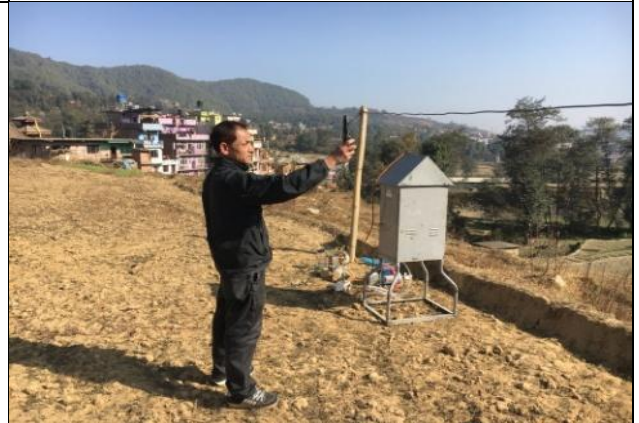
Photo 28. East Portal Wind speed & Temperature Monitoring
