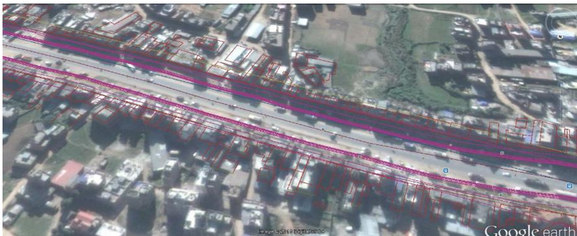
Figure 7.9-1 Alignment with Reduced RoW at Banepa Area
