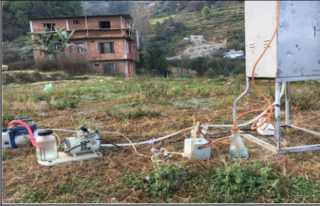
Photo 25. West Portal LVAS along with Gaseous pollutant Monitoring
