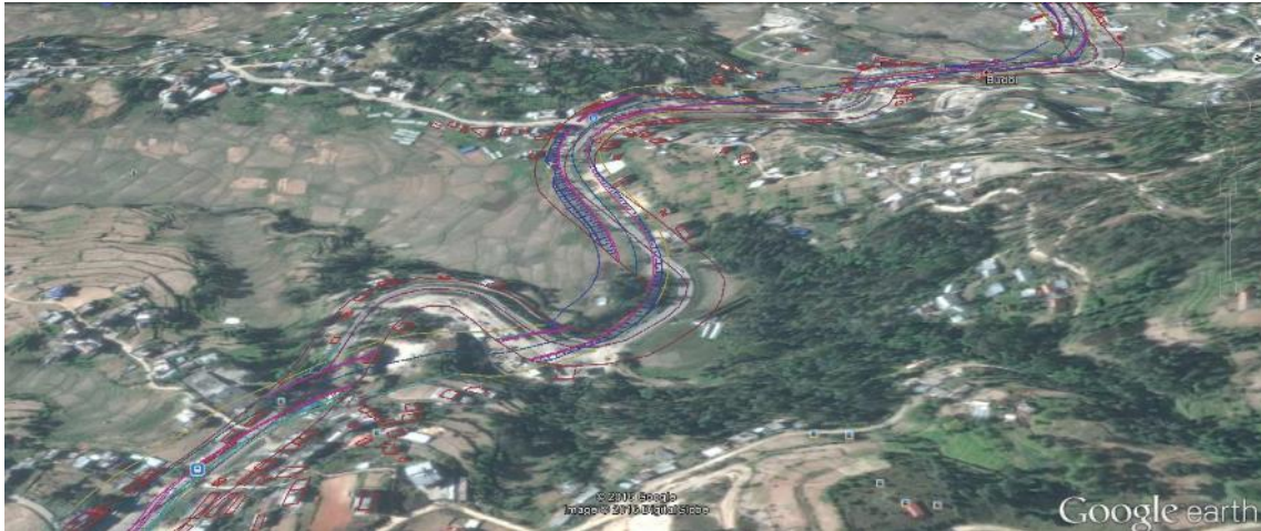
Figure 7.8-1 New Alignment with Improvement of Sharp Curve at Dhulikhel and KU Chowk
