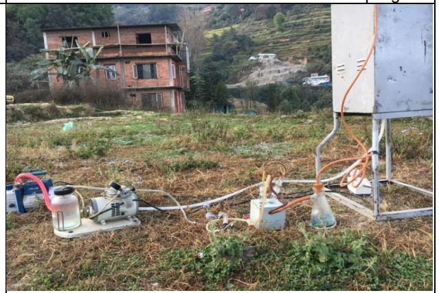
Photo 32: Air Quality Sampling at West Portal
