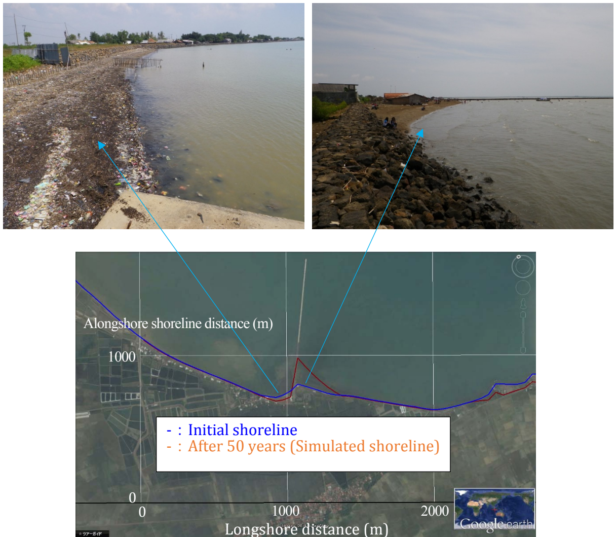
Figure 3.41. Predicted Shoreline Around the Existing Jetty After 50 Years with the New Port
