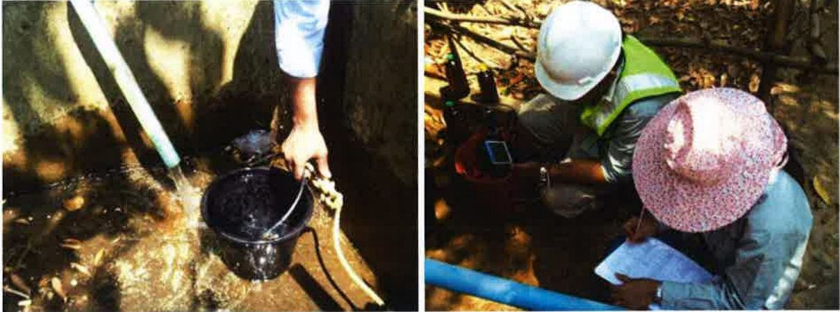
Ground water sampling and onsite measurement at GW-1
