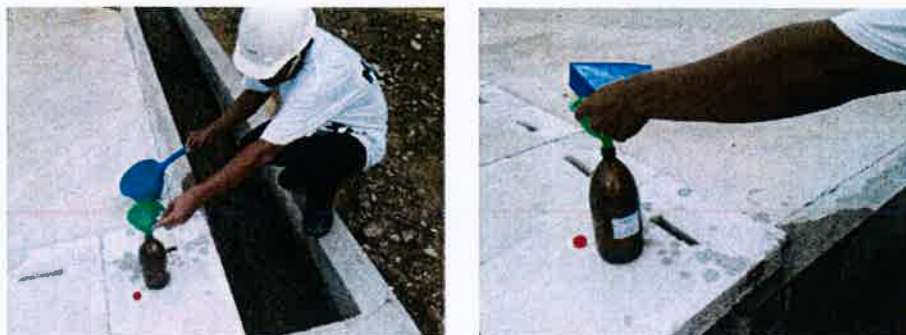
Figure 2 Sample Collecting at Sewage Treatment Plant (STP) Outlet
