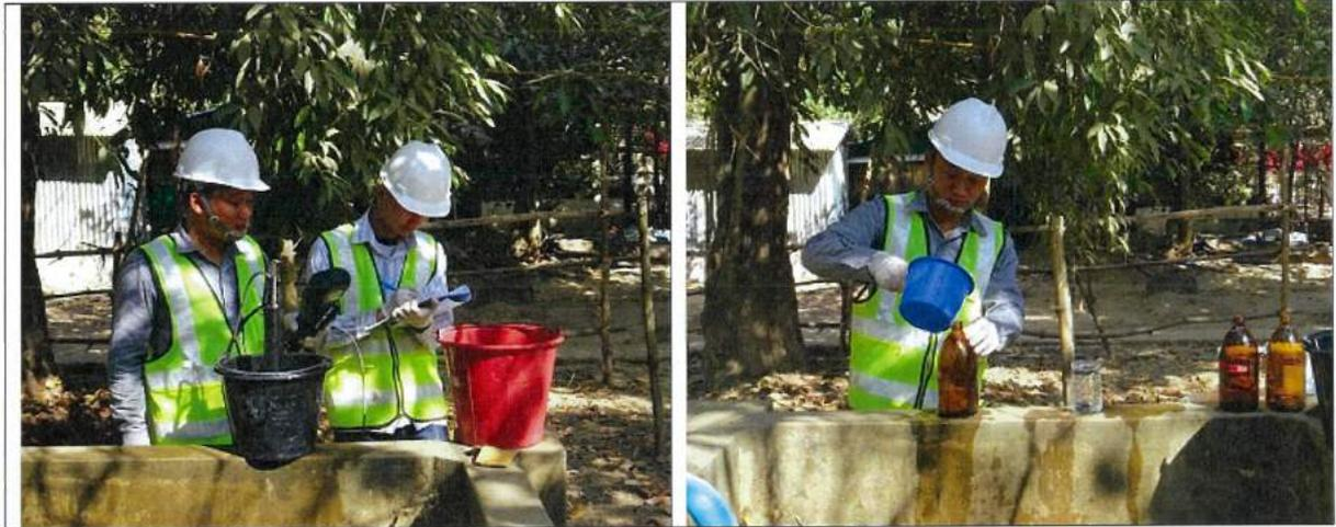
Ground water sampling and onsite measurement at GW-1
