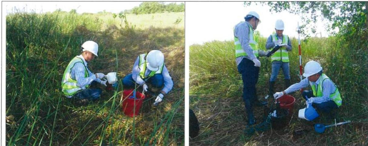
Surface water sampling and onsite measurement at SW-3
