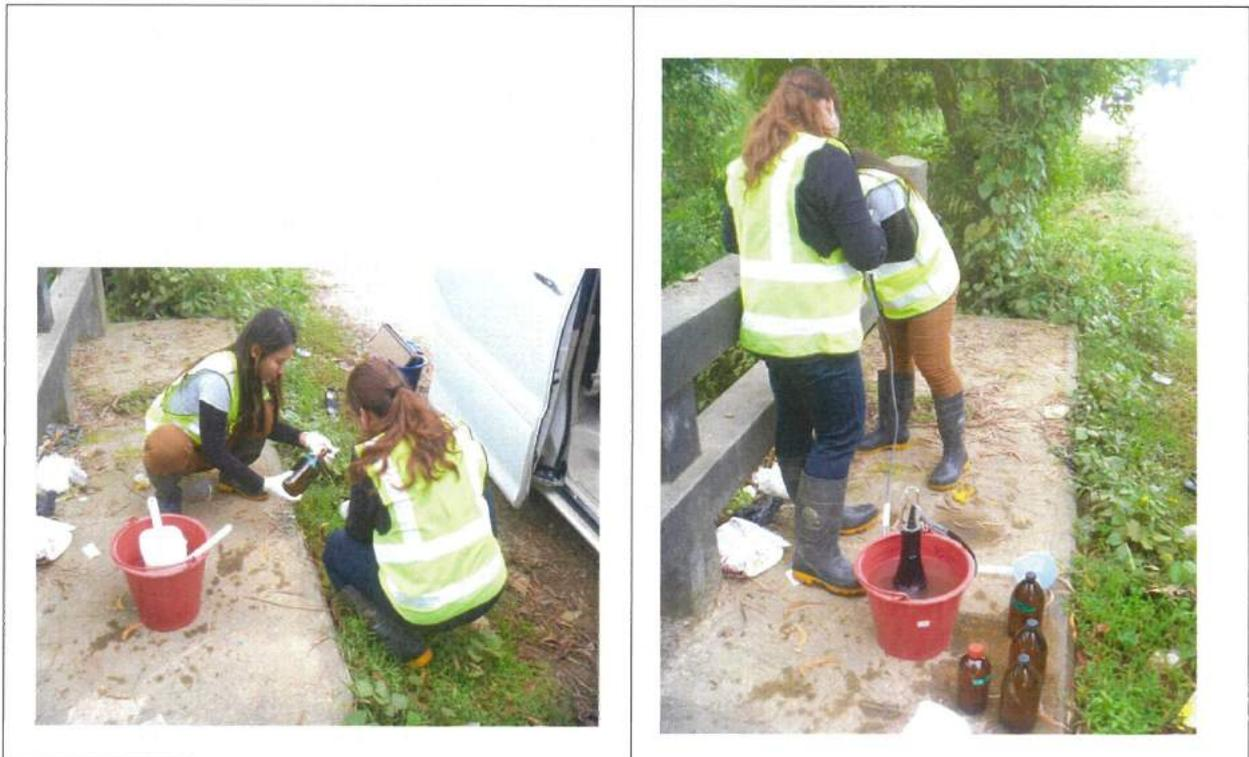
Surface water sampling and onsite measurement at SW-2
