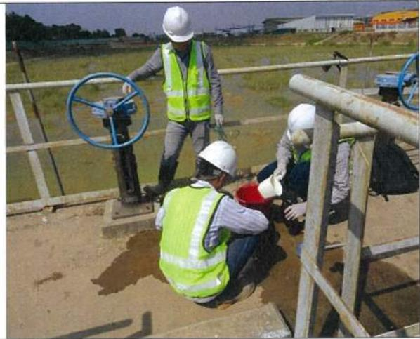
Surface water sampling and onsite measurement at SW-1
