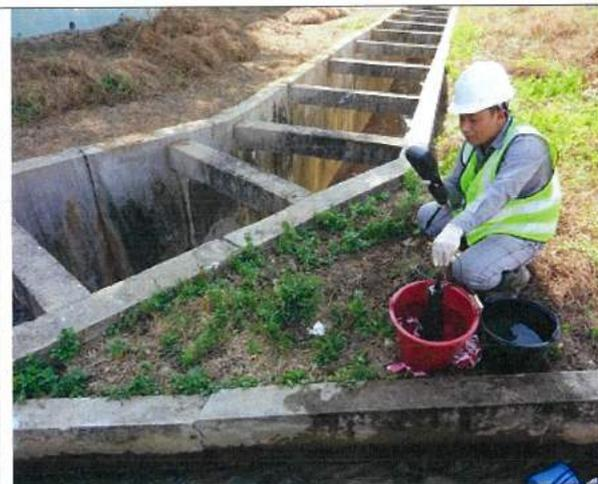
Surface water sampling and onsite measurement at SW-6
