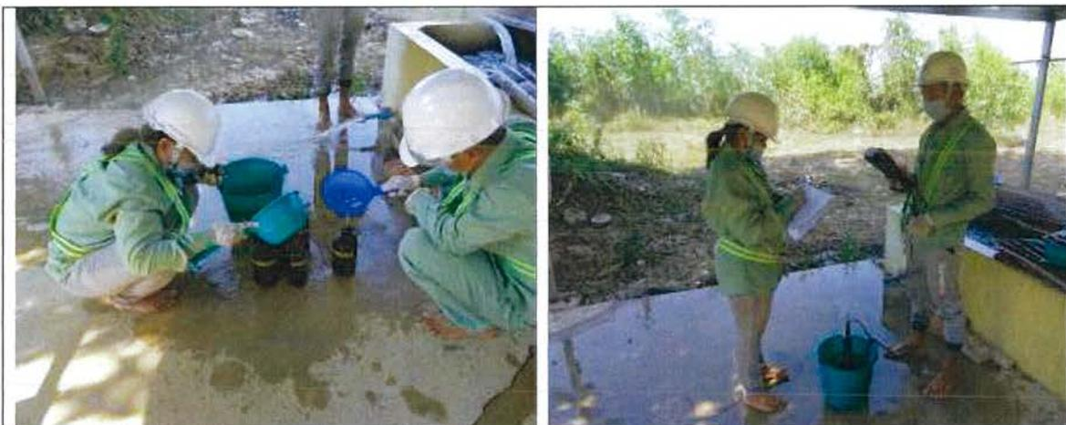
Ground water sampling and onsite measurement at GW-2
