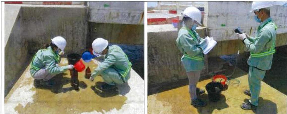
Surface water sampling and onsite measurement at SW-4
