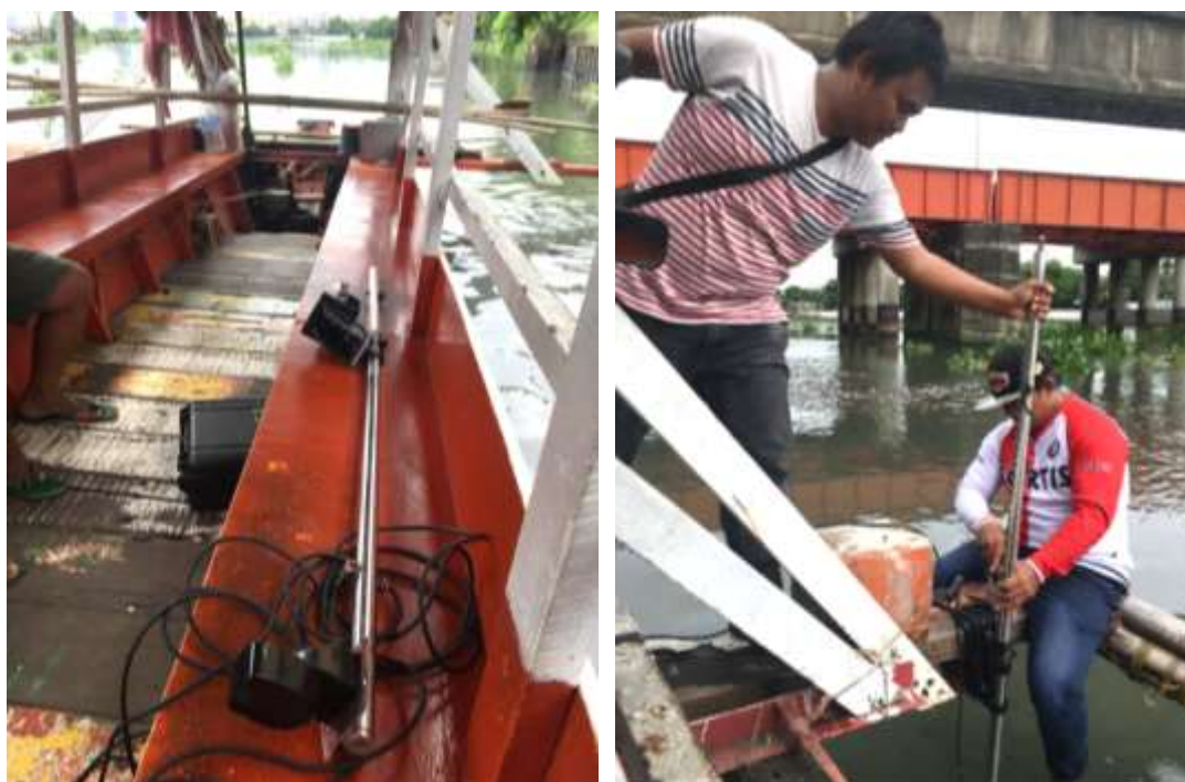
Figure 4.2.123 Major equipment installation status (echo sounder)
