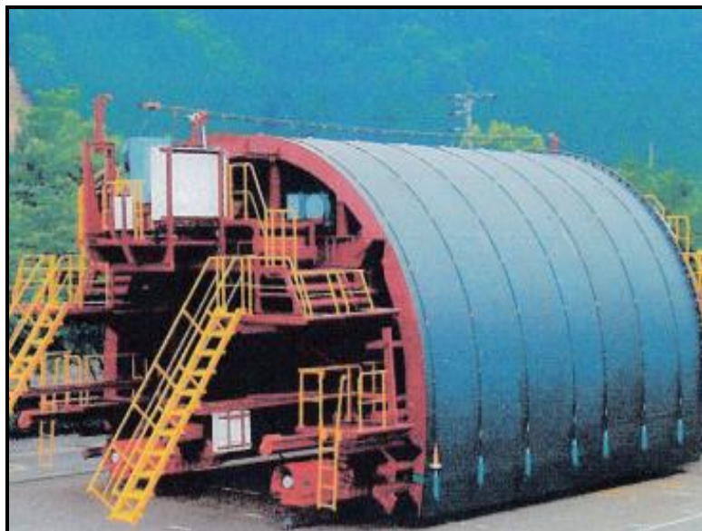
Photo No. 1.5.3-2 Sliding Steel Form ( Source: JICA Study Team, July 2014 )
