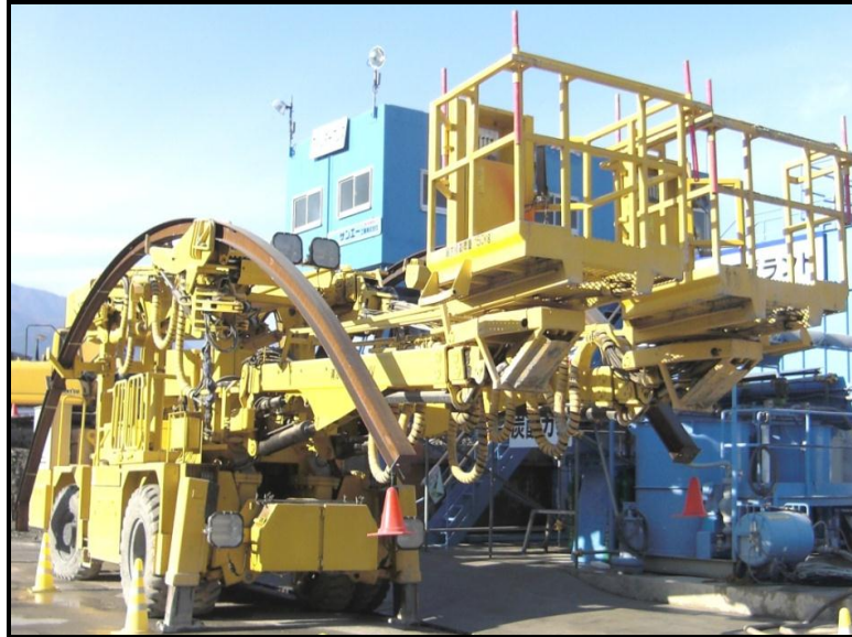
Photo No. 1.5.3-9 Steel Supports Setting Equipment (Source: JICA Study Team, July 2014)
