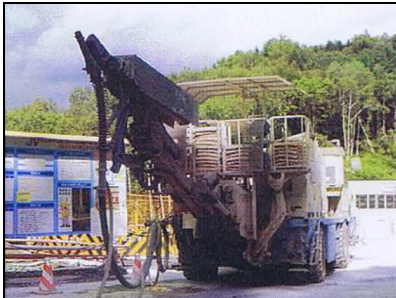
Photo No. 1.5.3-4 Shot Crete Machine (Source: JICA Study Team, July 2014)
