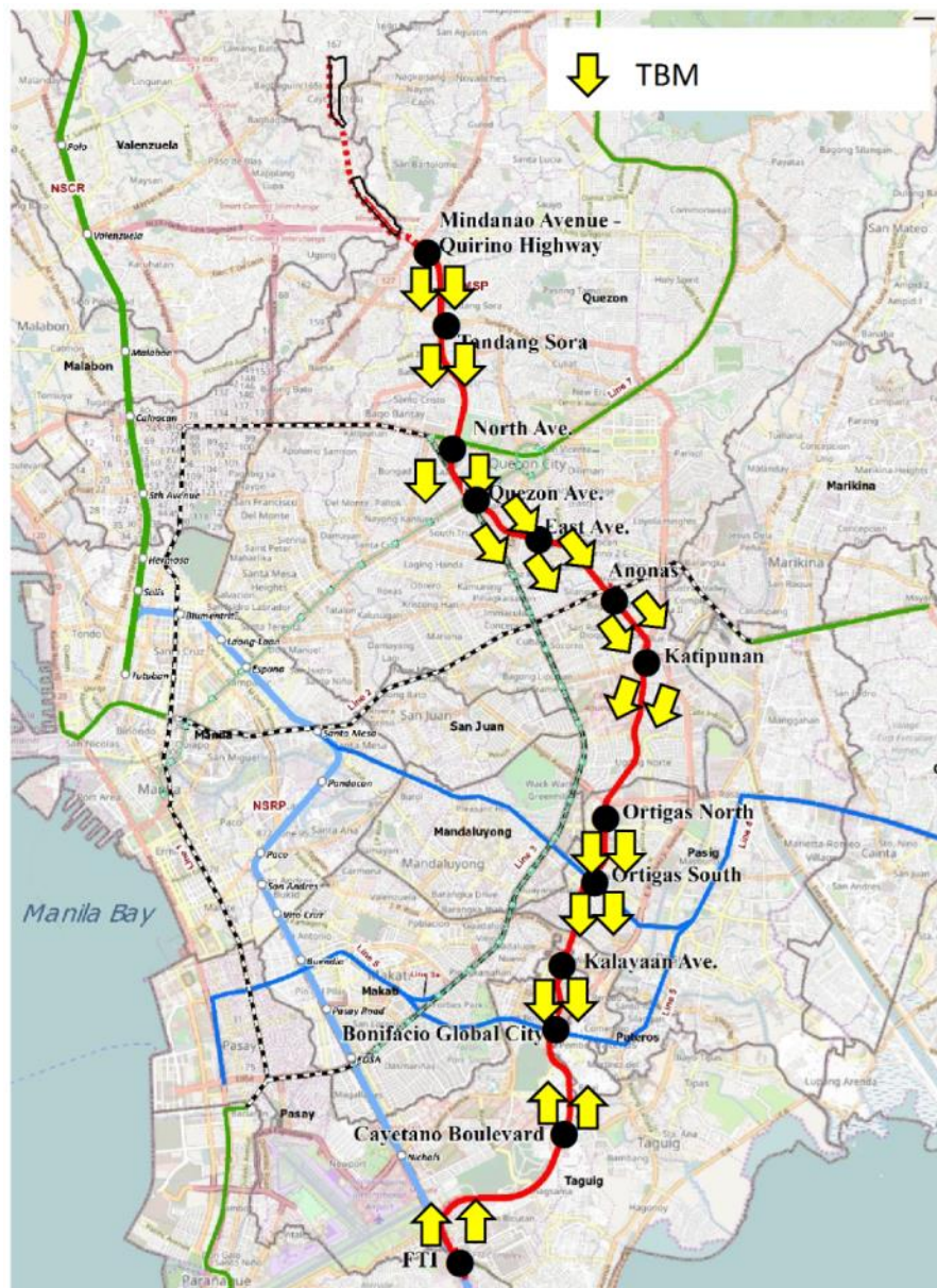
Figure 10. Typical TBM Operation Scheme Shielded Tunnel Excavation Planning
