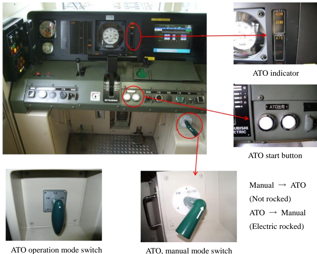
Figure 4.3.27 Sample of ATO·PSD switch (Tokyometro, 10000 series)
