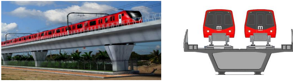
Figure 1-3. PC segmental box girder
