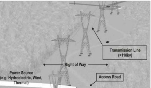
Figure 103: Right of Way and Access Road for OHTL (IFC, 2007)
