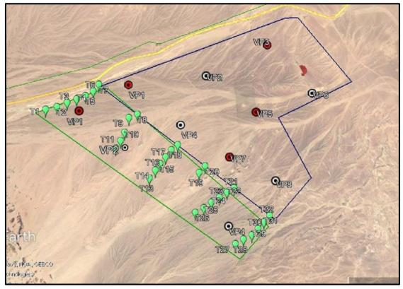
Figure 83: Location of Infinity I (200MW), green outline and turbine layout, and its neighbouring project (500MW), blue outline and respective VPs.
