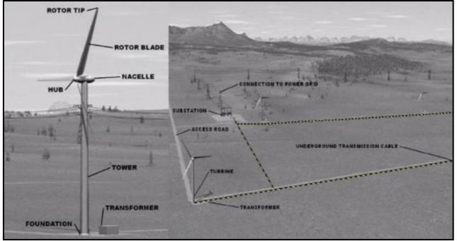
Figure 9: (a) Typical Structural Components of a Wind Turbine, (b) Typical Components of a Wind Farm (Source: EHS Guielines for Wind Energy, IFC)
