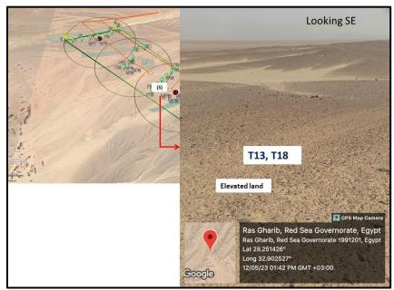
Figure 45: The area where the turbines T13 to T18 are located. Note the very weak drainage lines without any sign of sever surface runoff.
