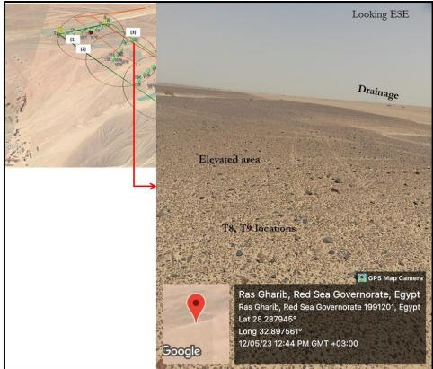
Figure 43: The elevation difference between the floor of the drainage lines and the next elevated areas where the turbines T8 and T9 are located. Note the difference is about 0.5 to 1 m at the east of the site.
