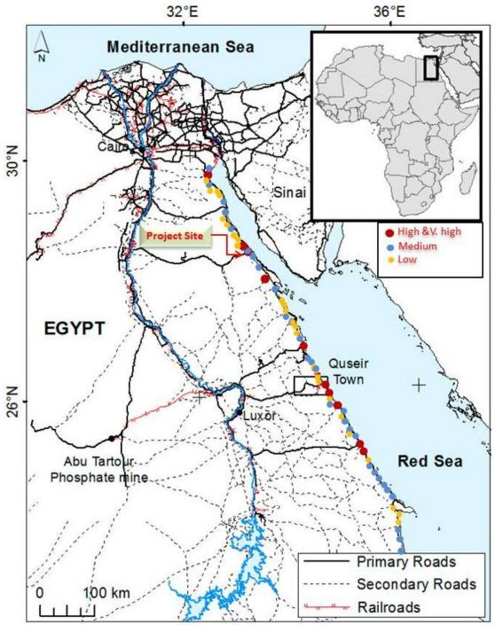
Figure 37: The likelihood flooding of the Red Sea area based on the historical record of the flash flooding.
