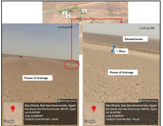
Figure 41: The elevation difference between the floor of the drainage lines and the next elevated areas where the turbines located.
