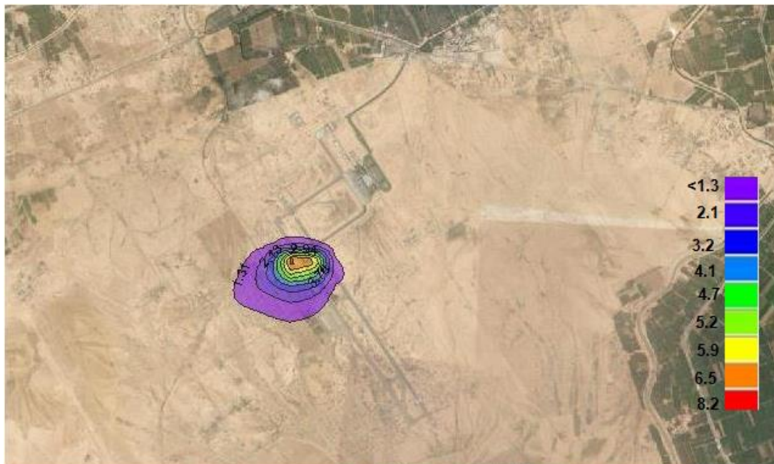
Figure (5-23) a predicted maximum annual average (SO 2 ) all over Borg El-Arab Airport Area.
