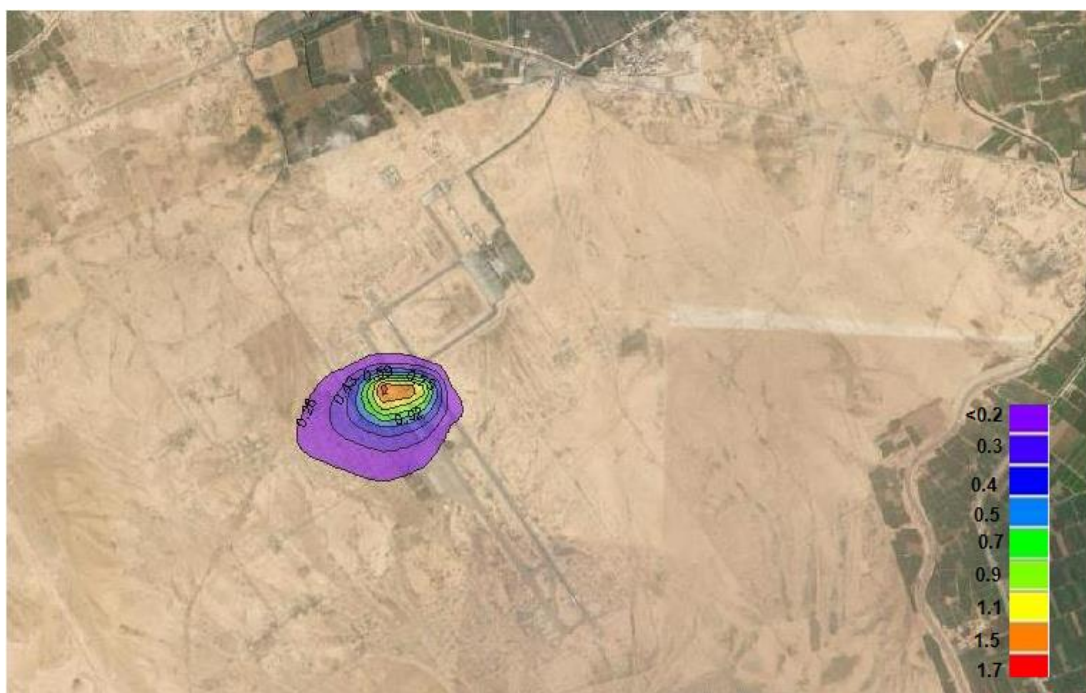
Figure (5-20) a predicted maximum annual average (NO 2 ) all over Borg El-Arab Airport Area.
