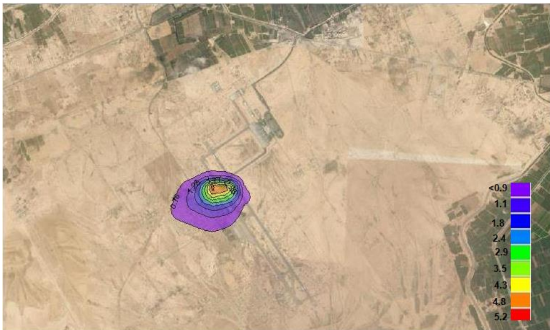
Figure (5-17) a predicted maximum annual average Carbon Monoxide (CO) all over Borg El-Arab Airport Area.
