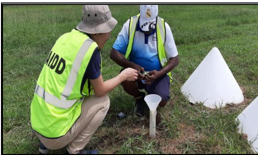
Photo 56 and Photo 57 Showing team placing the filter paper in a funnel to collect air particulates in the filter paper and the dissolved solids in the rainwater in the funnel.
