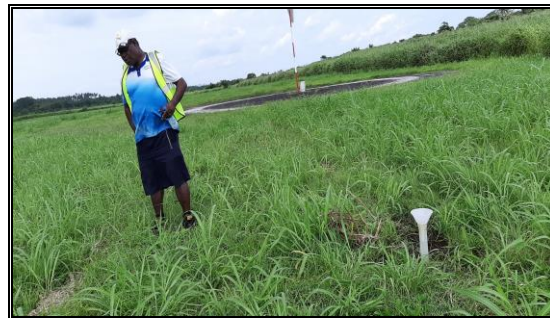
Photo 56 and Photo 57 Showing team placing the filter paper in a funnel to collect air particulates in the filter paper and the dissolved solids in the rainwater in the funnel.
