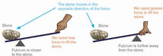
A lever is a very useful simple machine. We can find levers everywhere. Examples of levers are flip top and shovel.
