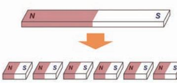
We can make many smaller magnets by cutting the big magnet
