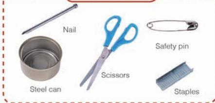
A steel can is attracted to a magnet, but an aluminium can is not attracted to a magnet. Why?
