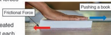
Frictional force: A book sliding on the table is creating an opposite direction of force.
