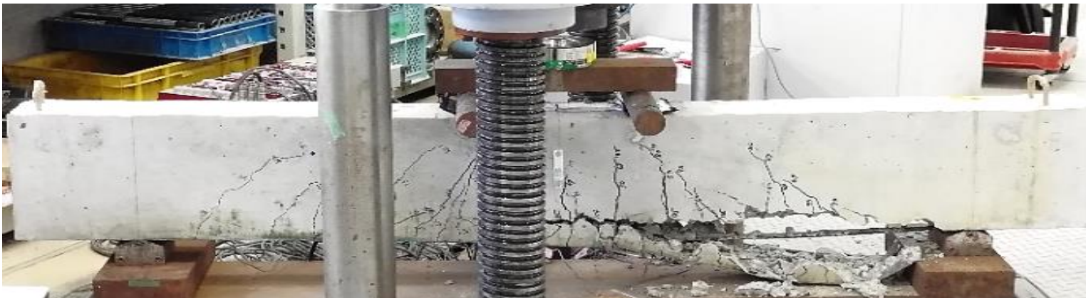
HS8F1 Failure modes=CS Crack nos.= 22
