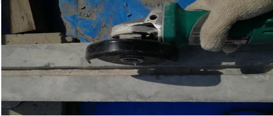
Fig: Making groove and grinding bottom soffit of specimen
