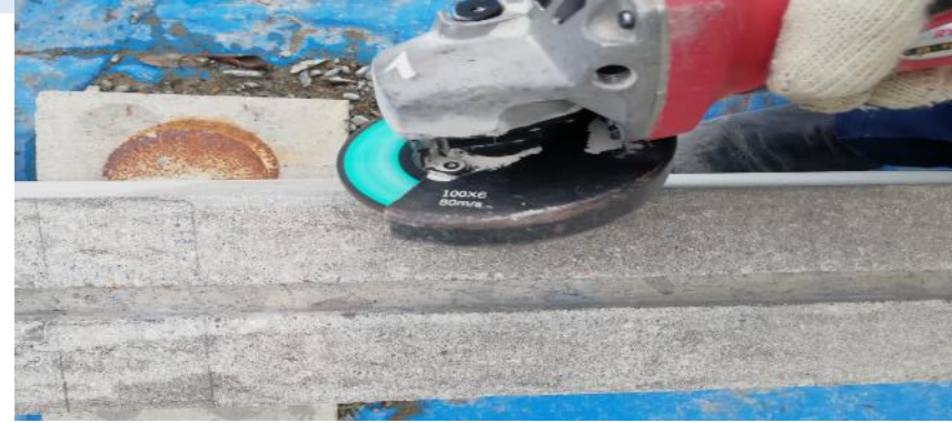
Fig: Making groove and grinding bottom soffit of specimen
