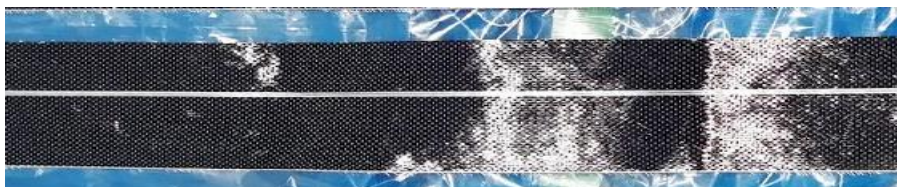
Fig: CF RTS Fabric (t=0.167 mm )
