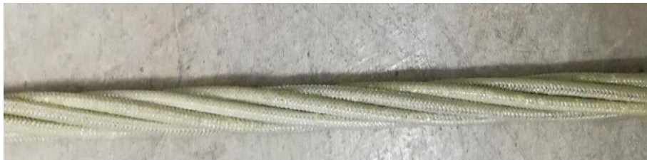
Fig: CF RTP bar( \varnothing = 9.3 mm)
