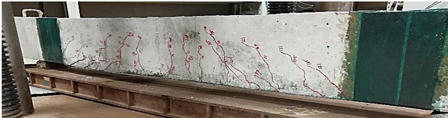
HP9F2A Failure modes=CS Crack nos. =22
