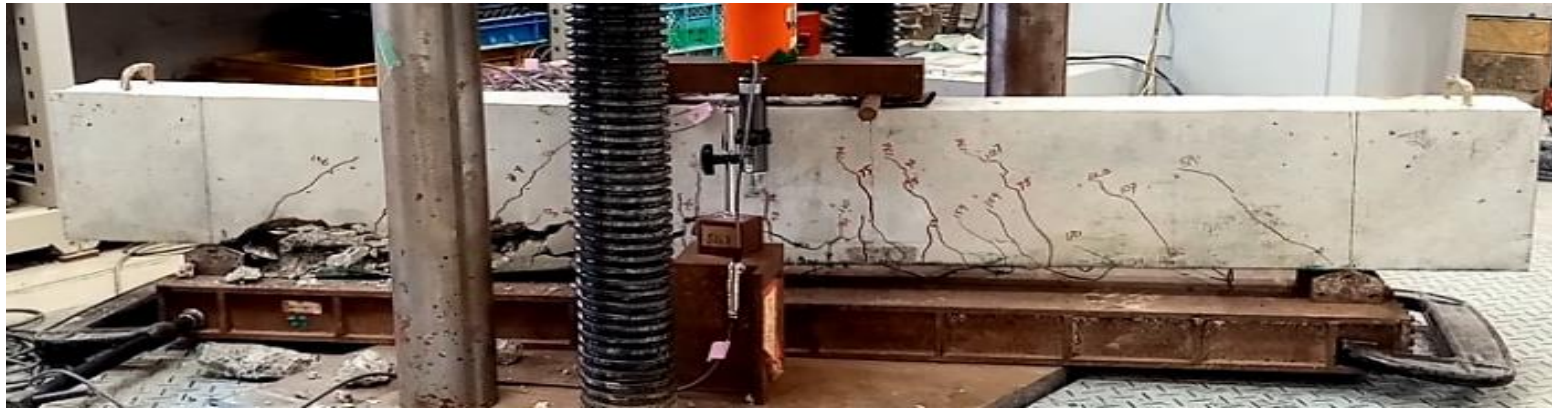
HP9F2 Failure modes=CS Crack nos. =24
