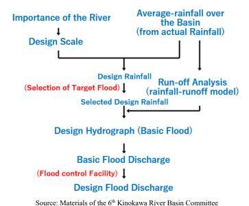
Figure 2.2 Design Flood and Basic Flood Discharge
