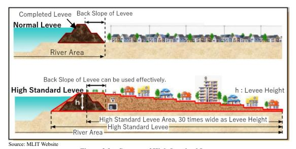
Figure 2.9 Concept of High Standard Levee
