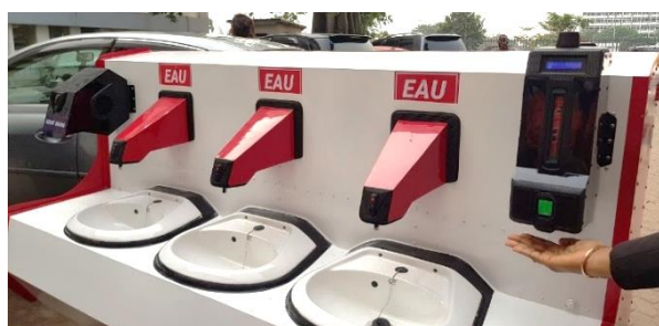
A thermometer/counter/liquid soap server (right), faucets (center), and a dryer (left)
