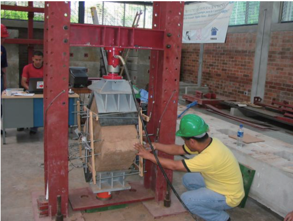
Diagram 2: Photo showing the experimenting on the seismic capacity of a brick
