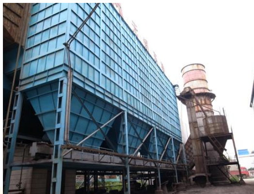
Electric dust collector installed into Steel Plant
