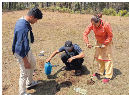
Hydraulic conductivity test to identify the depth of the pond to be renovated in Syangja.
