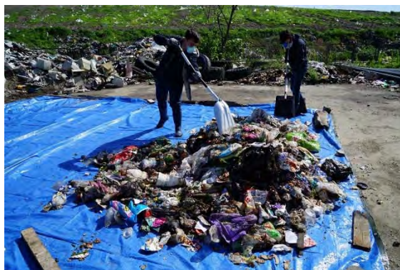
Mixing (waste in plastic bags was taken out and all the waste was mixed well)
