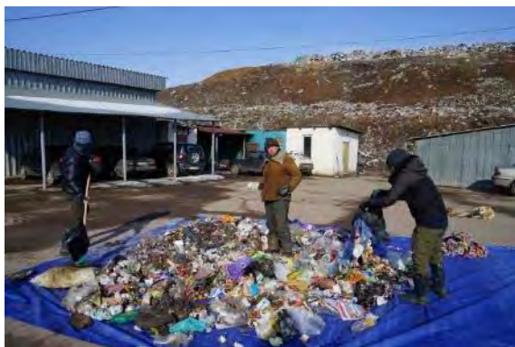
Target waste (over 200 kg of municipal waste was taken from waste collection trucks)
