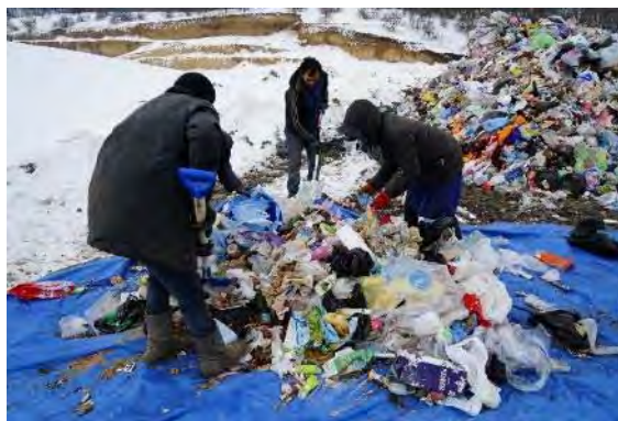
Mixing (waste in plastic bags was taken out and all of it was mixed well)
