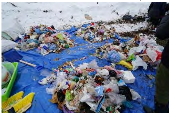
Conical quartering (over 50 kg of waste remained for segregation)
