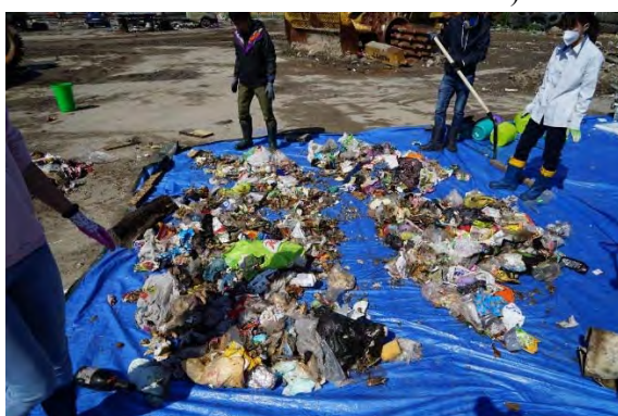
Conical quartering (over 30 kg of waste was remained for segregation)
