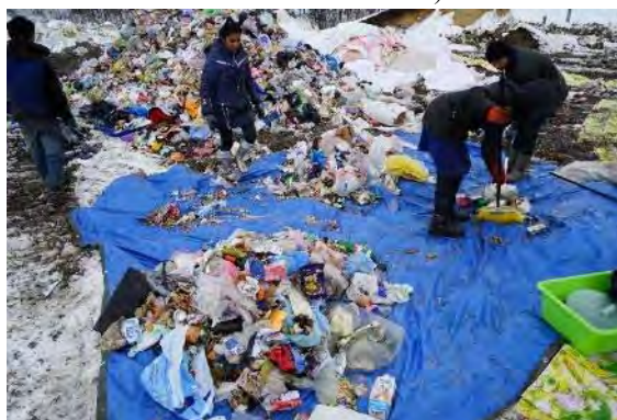
Conical quartering (over 50 kg of waste remained for segregation)
