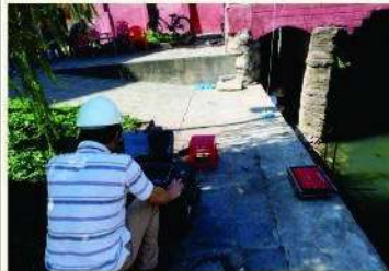
Measuring the vibration of monument
